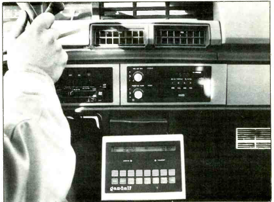
This is the passenger's view of a taxi equipped with Gandalf Technologies' computerized dispatch system. The cab driver communicates with the cab company's dispatch center by pressing various buttons on the mobile display terminal. The driver also receives calls via the terminal. (Photo courtesy of Gandalf Technologies, Inc.)
