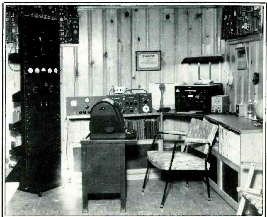
An old-style RTTY station using the bulky equipment that has mostly been replaced by modern technology. This stuff clattered away and sounded like a Thompson submachine gun!
