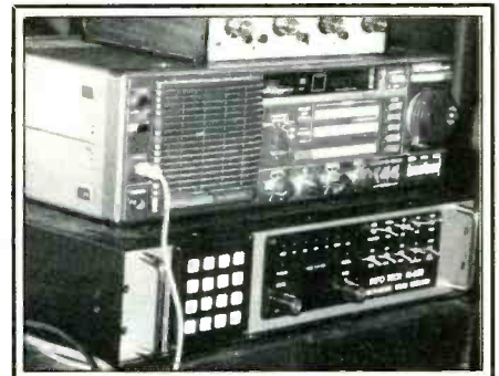
At the bottom of this stack of gear is an Info-Tech M-600 multi-mode RTTY decoder, one of the more sophisticated units available to the monitoring enthusiast. It's capable of unraveling RTTY/ARQ/FEC and even CW. It also cracks "bit inversion" privacy codes!
